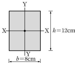
$$\begin{aligned} \bullet I_X &= \frac{bh^3}{12} = \frac{8 \times 12^3}{12} = 1,152 \text{ cm}^4 \\ \bullet I_Y &= \frac{hb^3}{12} = \frac{12 \times 8^3}{12} = 512 \text{ cm}^4 \\ \therefore I_X &> I_Y \end{aligned}$$
